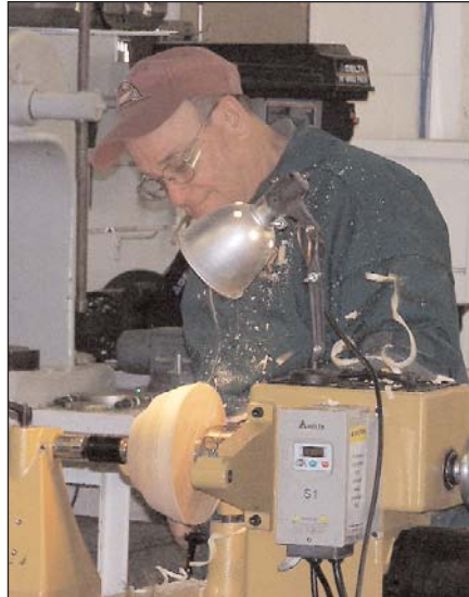
Working fast to minimize heat build-up and to avoid excessive reshaping that would be needed after warpage.
