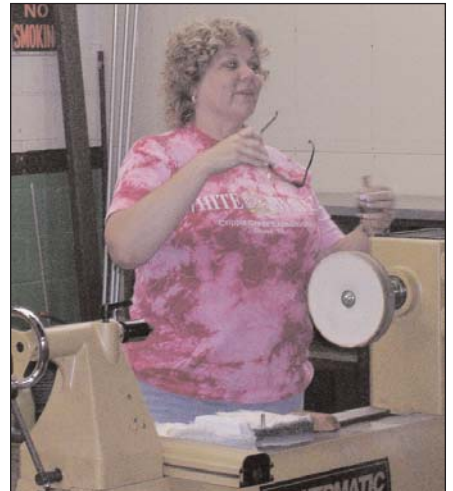
Denise Milstead demonstrating the use of the Beal Buffing System to produce smooth projects with varying degrees of sheen.
