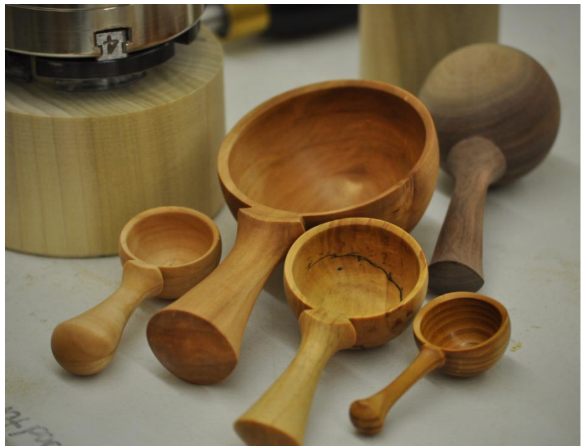
Four finished ladles. The walnut piece is ready to mount in a jam chuck to hollow out the bowl.
