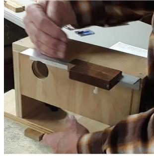
Shown at right is part of the glue-up jig Mikeal uses to space and glue in place the segments used in a bowl blank.
