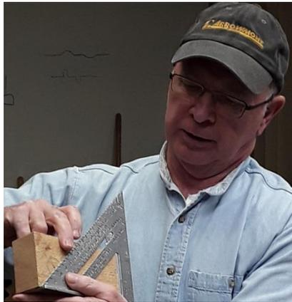
The first step was to locate the “ball” position on the wood blank. This is necessary to help keep the board turning true by placing both centers equidistant on the blank.
