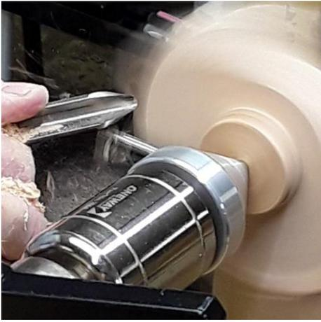
As turning commenced, the obvious “air” turning began. From a thick board came one that was much thinner with a “knob” on both sides where the “ball” would develop.
