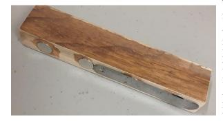
This is a detail of the positioning fixture with magnets to hold the angle disc (*red disc on page 3 and 4*) in place for segment positioning. Made of hardwood with an indexing hole (*right*) and magnets glued to it, it is stuck on the headstock. Aluminum lathes need a steel plate fastened to allow the fixture at left to be positioned.
