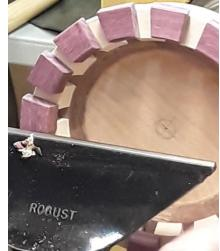
All open segments have been placed on this form. The next layer will be a solid layer to tie the open segments together and provide a smooth top surface. Notice the pattern of segments as seen on the inside.
