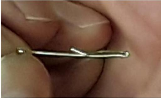
The Clapper wire was made into a clip of sorts. This clip was then pushed into the top of the clapper and then the hanger wire was attached and pushed through the top of the bell turning.
