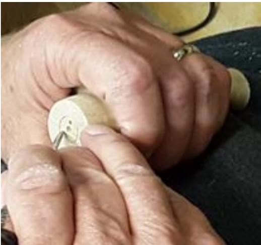
To enable the off-center turning process a series of three center locations were marked on the tailstock end of the turning piece. The ring mark made by the dead center became the locating position for each of the off-center locations, hence the term off-center turning.
