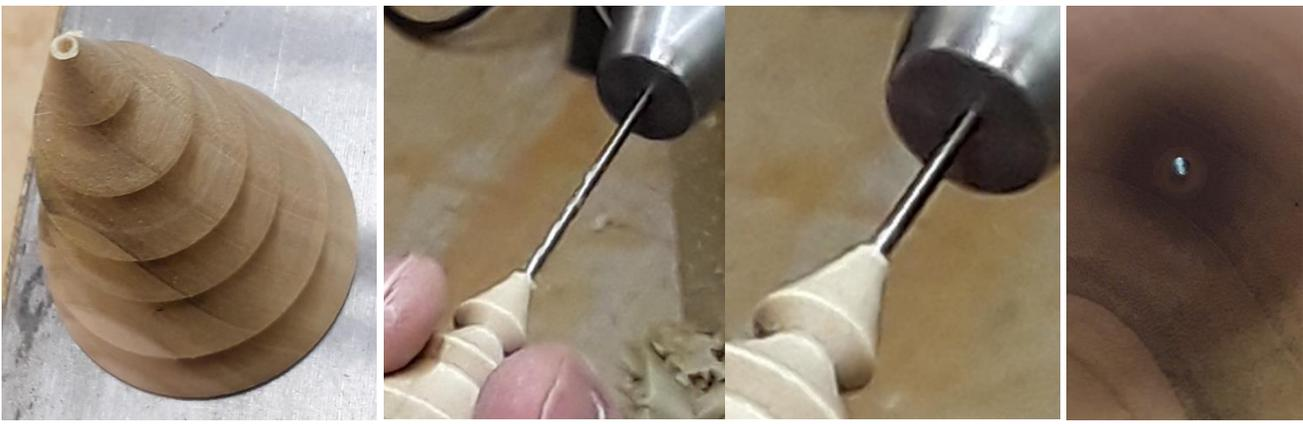
Harlan then turned his attention to the clapper. Below is the progression from square stock to parting off the finished clapper.
