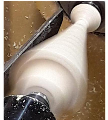
Shown below is the progression on the first “off-center” location. These slits will be colored on the finished turning. Note that only every fourth line has been turned so far. Each successive center will locate another set of slits one-third of the way around the “tree.” Depending on which way the off-centers are chosen will determine the progression around the tree as one goes up the turning.
