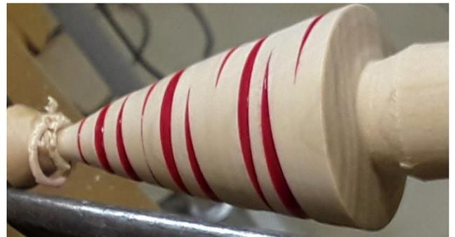
After slitting each of the three off-centers, coloring the slits with a permanent color, and turning the final smoothness, the tree is ready for finish turning.
