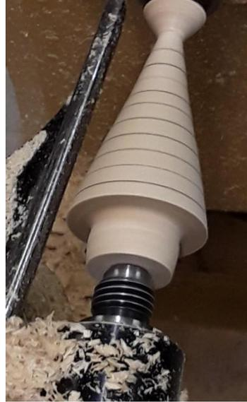
Once the shape progressed, lines were marked at regular intervals. These lines would become the spots where the offset turning would be done. Slits would become design elements in what would be a small tree-shaped ornament.
