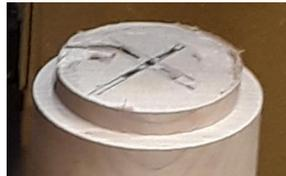
Then the "pusher is laid out for a push stick made from a 5/16" dowel rod. The pusher is reduced in diameter to at least 1/2" smaller than the inside of the cutter,
