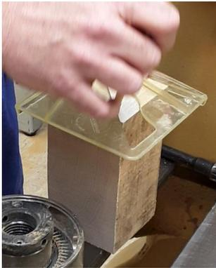
Next, a center finder was used to locate where to put the centers on the lathe.
