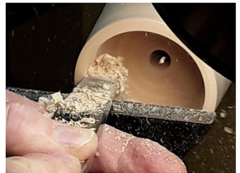
Progression from removal of the “pusher to layout of the cutter to interior shaping progresses. Since the biscuit size will be 2” the inside must be turned to approximately that size. Depth must allow for the pusher as well as the maximum thickness of biscuit dough—about  $\frac{3}{4}$ ”.
