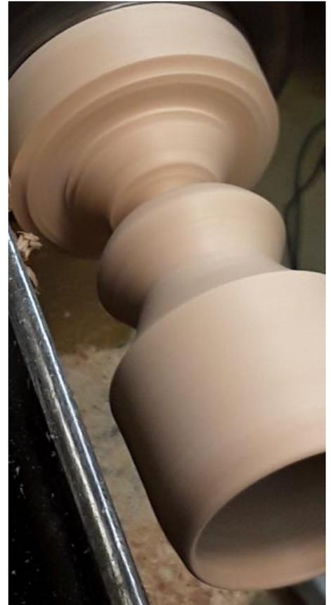
Once the interior is shaped, sanded smooth and drilled for the pusher handle, the final shaping of the exterior is done. Last step after sanding the exterior is part-off the finished cutter.
