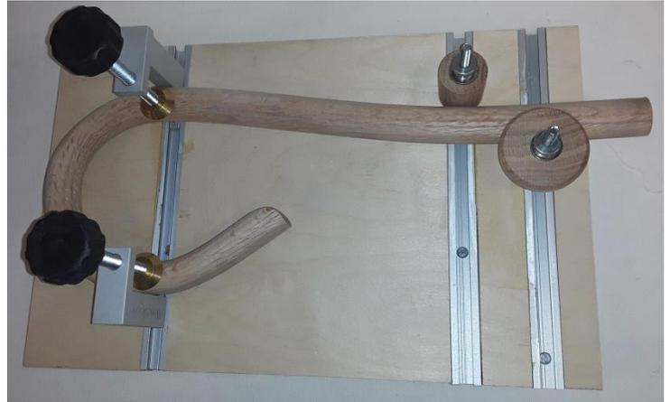
Club Treasurer **Chip Sisky** brought a fixture he uses to produce the crook at the top of the staff he produces for Bishops worldwide. The fixture is adjustable for several reasons: **a.** to allow insertion of the softened staff crook and **b.** to provide for any variations in design of the crook based on diameter of the stock. On VERY close examination of the crook Chip brought, a small crack can be seen on top of the crook.
