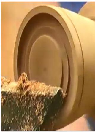
Changing from a parting tool to a beading/parting tool David began to establish the interior hollow of the egg part.
