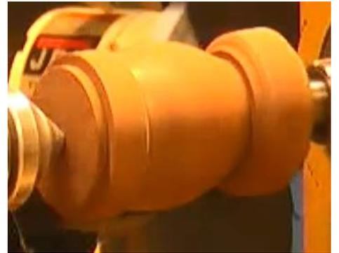
The progression from round to rough egg shape is shown above. The largest diameter is approximately in the “center” of the egg.
