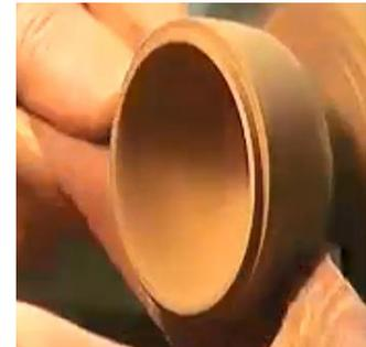
Final shaping of the top of the egg can be seen in the pictures above along with some finish sanding of the outside surface. Now all that remains is to release the egg half from the “pud” in the chuck.
