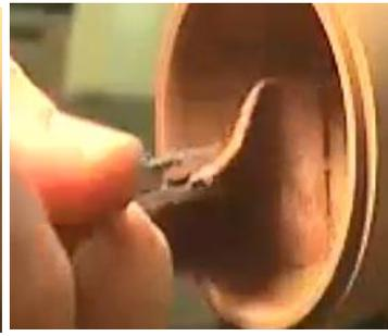
Some light sanding using a “finger-saver” finishes the inside of the 2<sup>nd</sup> half of the egg. One quick touch to the end of the egg assures a good, tight fit when the two halves are re-assembled.
