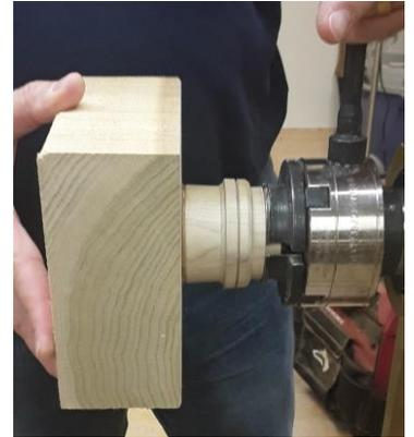
This was reinforced with a small bead around the outside of the chuck mount where it met the block. Then the assembly was mounted in the lathe chuck and securely tightened. A mark was put on the chuck mount where jaw #1 was in case of needing to remount later.
