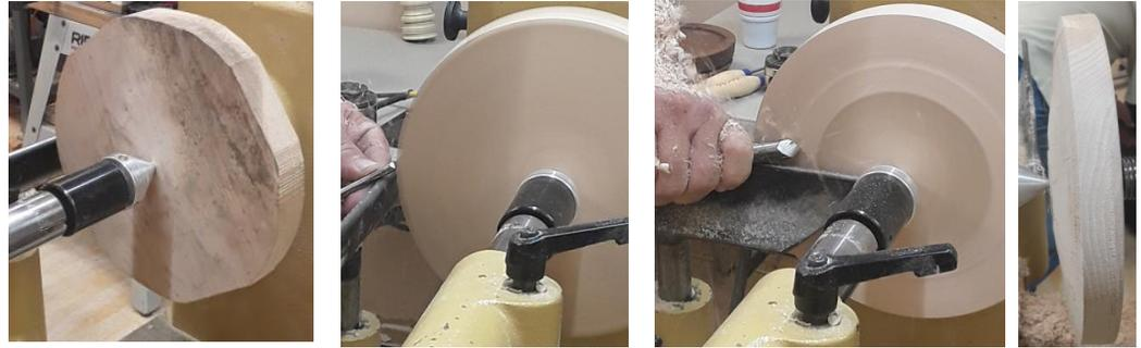
From this a slight indentation was turned to allow mounting in the chuck when turned around. (*see below*)
