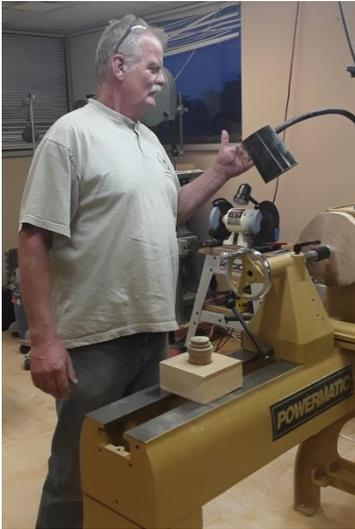
The feature for September was a plate turning by VP Danny Smith. Beginning with a slab of Maple about 2" thick Danny first trued it in the lathe between centers. This was after approximating the center on each side. The next step was to true the side away from the headstock and turn a slight taper to this side. Note the progression below.
