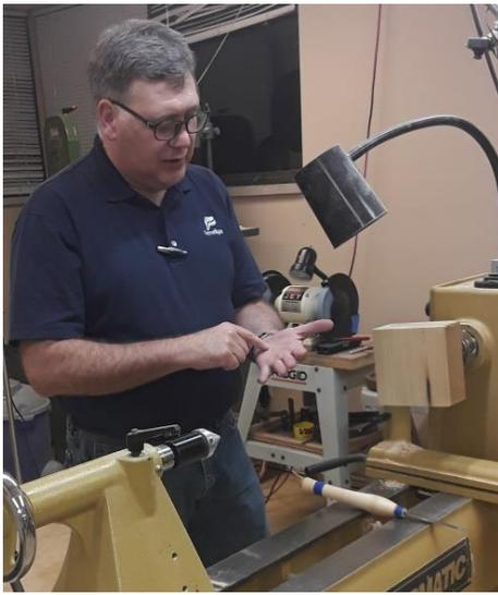
Now for the “Two-fer” demo. Chip Siskey showed the process for making a backing block or how to turn a blank without putting an inset to mount in a chuck.
