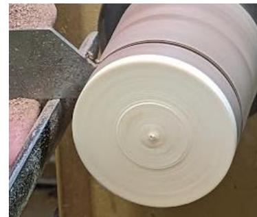
From Left to right above, David first turned the cylinder round using his “giant” roughing gouge. Then laying out for a tenon on one end that will be clamped in a chuck, David proceeded to turn the end. After that, the throw-away of the box was cut off with a thin parting tool. The top is still attached and in the chuck
