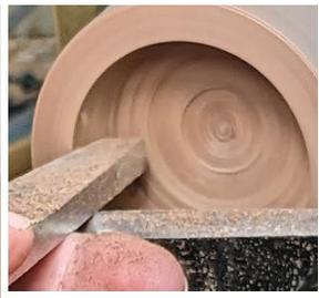
Using a bowl gouge, David hollowed the end of the box to the approximate depth needed. Changing to a **Bedan** tool, which has a heavier shape and is made for squaring the bottom of a hole, David smoothed the inside of the box to final shape.
