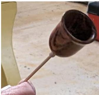
Jim Tate brought a long stem “goblet” made with Hard Maple. The stem is about 1/8” in diameter and turned in one piece and then assembled to the cup and base. Total height is about 12” overall.
