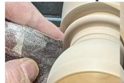
This is the best time to do sanding on the exterior of the ring before it is released.
