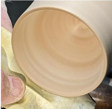
Note the smooth transition from side wall to bottom using the carbide insert tool as shown at the left. Once the basic shape is attained, the “boring” job of sanding takes place.
