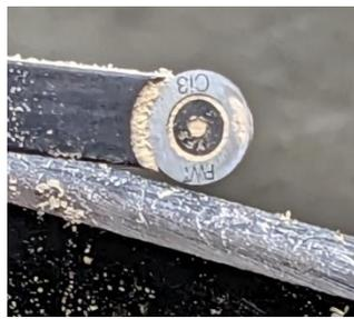
Once David began to turn the inside of the goblet, he switched to a carbide tipped tool because of the smoothness of the resulting turning. Sharpening is eliminated—just turn the insert a little to expose a new edge.
