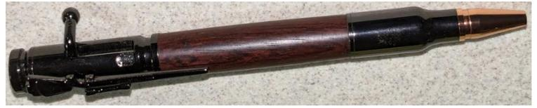
The second pen below is made with **Honduran Rosewood** and is a bolt-action ballpoint pen. It uses a different refill and is drilled with a 10mm drill bit. It is finished with **Walnut Oil** wax.
