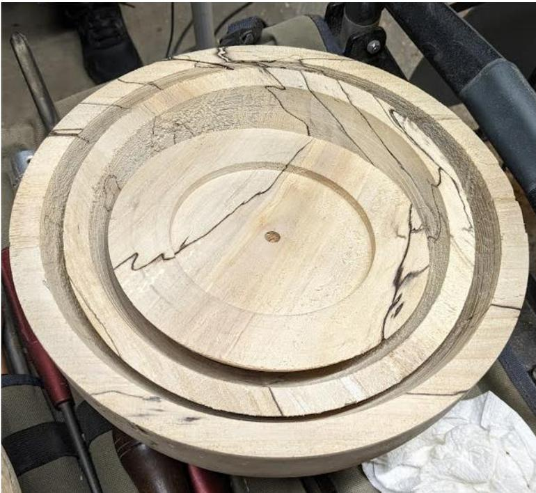
Minimal waste wood was generated in creating these three blanks. A finished set of bowls from this process could bring as high a price a \$200 to \$300 depending on the type of wood being turned.
