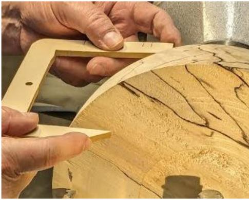
Alex also has a set of “helper” measuring tools to determine where the inside of the largest bowl will be. This insures that a “funnel” isn’t the result of turning the wood
