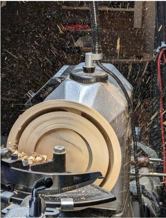
Chips fly as the tool proceeds into the bowl blank and as the far end of the cut is almost completed. Safety is imperative when using this tool since, like other turning processes, chips can become dangerous if one's not careful.
