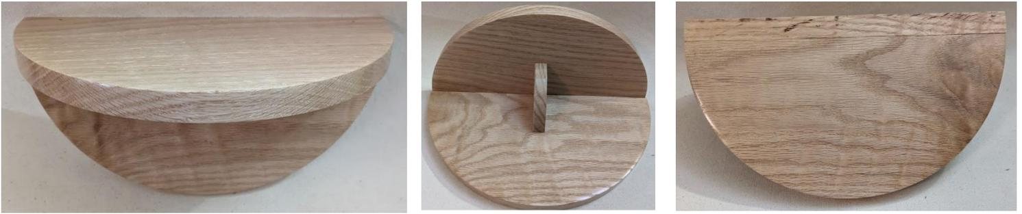
Treasurer Chip Siskey brought an Oak shelf that at first glance would not look like a turning. However, Chip's explanation cleared that up easily. Made initially as a round disc on the lathe, parts were then cut with the upright being slightly past center and a small Oak brace placed under the shelf which was the other part of the original disc. Finished in Lacquer, the hanging process for the shelf was not divulged.
