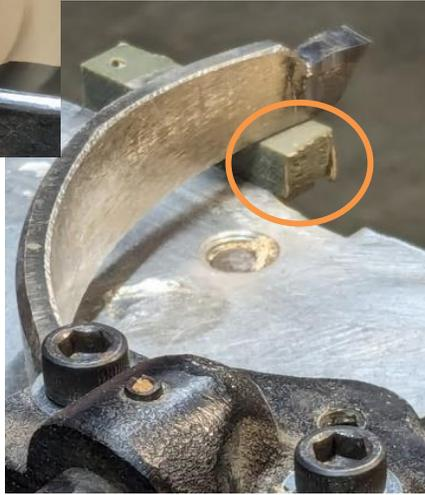
Note the block that is under the tool at left. This block is part of the tool but is not long enough to support the larger tool when making the first cut. Because of this, more noise is present; and more vibration is possible based on the type of wood being used and the speed of entrance into the turning.
