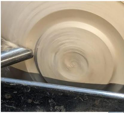
Turning the inner blank around, a tenon is cut into the base of the exterior to mount the blank back on the lathe using the One-Way chuck. This is to allow use of the *Woodcut Tools Ltd Bowlsaver* to extract the small bowl.
