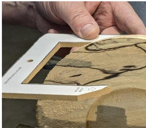
Once again the smaller of the two gages is used to determine the bottom of the bowl. These templates were originally on paper and Alex glued them to plywood, cut the plywood to form the gage to be used.
