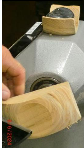
The prototype is seen with a bar of soap lying in the turned dish. Since it will be exposed to water when in use, super sanding is not necessary upon completion of the turning.
