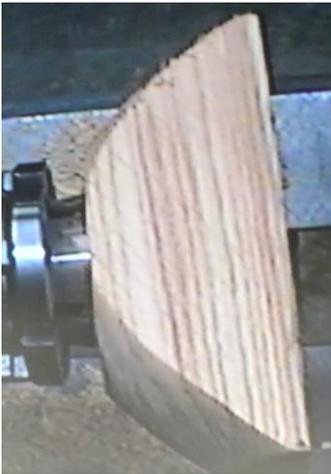
Block thickness can be seen at left for the external shape being turned. This is necessary to provide the depth on the finished turning to hold the soap bar.
