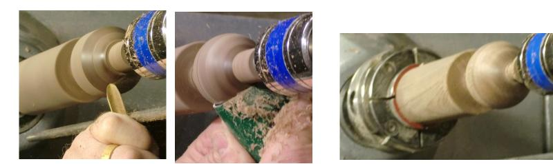
Using a spindle gouge Chip completed turning the bowl "ball" end first before shaping the handle. At the far right above the blank has been mounted in a One-Way<sup>™</sup> Chuck to hold the part for the next part of the shaping process.
