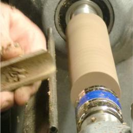
Once round, the bowl layout and marking is done using a dividers and parting tool to indicate what part to be left at this point. It's important to be sure not to cut too deep and cause weakness while turning the other details.
