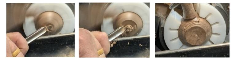
Using the bowl gouge, a hole surface is faced off first. One must be very careful to grip the tool firmly and present it correctly to the wood or what happened in the far right picture will be the result. Fortunately, no serious damage occurred and that part can be turned off in the final scoop.
