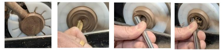
From the faced-off part a hole is started with the gouge. When enlarging the hole the angle of attack is very important. Once the hole is begun, cleaning and enlarging is commenced. One must make sure not to take the hole too deep or a nice handled-funnel will be produced. (Tee Hee).
