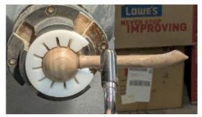
Here is the piece clamped in the chuck for turning the interior of the scoop. Note the clearance required for the handle to spin while turning takes place.
