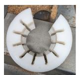
Formed from UHMW (*Ultra-High Molecular Weight Polyethylene*), this holds the bowl portion of the just-turned coffee scoop. The cuts are to allow some flex when being clamped in the One-Way<sup>™</sup> chuck.
