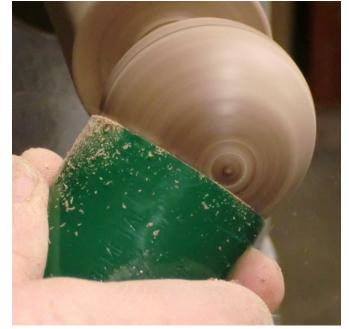
Turning the handle to size and leaving enough to offset for the design mentioned previously on page 2, the chuck is removed and the turning live center is reinserted in the head-stock. Moving the contact point over about a 1/4"-3/8" the blank is clamped between centers and a fingernail-grind spindle gouge is used to form the offset turned part of the end of the handle.
